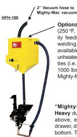
Optional HFH-100 heated hopper (250 °F, 121 °C) automatically gravity feeds recovered flux to lower welding system hopper. System available with magnetic separator, unheated and in different flux capacities (i.e. 200 lbs, 300 lbs, 600 lbs, 1000 lbs etc.). Must be used with Mighty-Mac vacuum.
